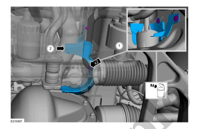
5. Disconnect the front differential breather hose and position aside.
