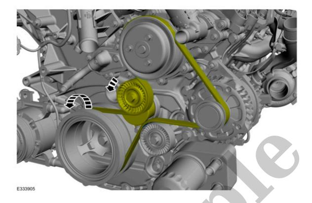
3. Remove the bolts and the accessory drive belt tensioner.
