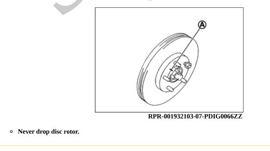
7. Using lock nut chisel (SST: KV40108800) (A), release staked area of wheel hub lock nut.
