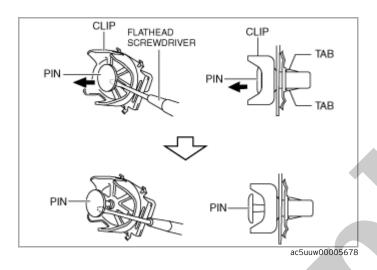
2.Insert a tape-wrapped flathead screwdriver into the positions of the arrows shown in the figure.
