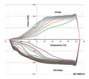
For optimal performance, cell operating temperature range is 10° C (50° F) to 38° C (100° F).
