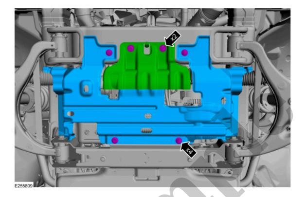
4. If equipped, remove the bolts and the skid plate.
