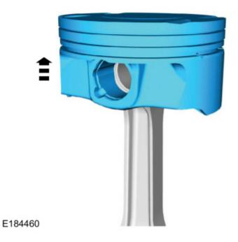
4. Clean and inspect the piston and connecting rod.
