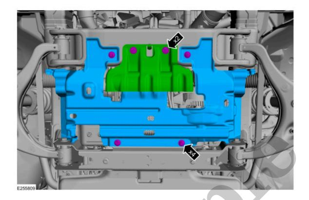
4. If equipped, install the transmission housing cover and the bolts
