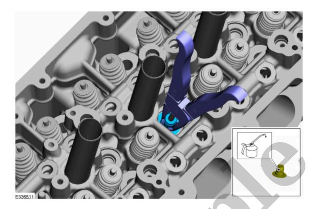
3. Using the special tools, install the spring, retainer and keys.
