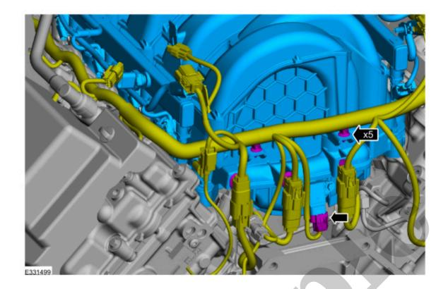
33. Tighten the intake manifold bolts.
