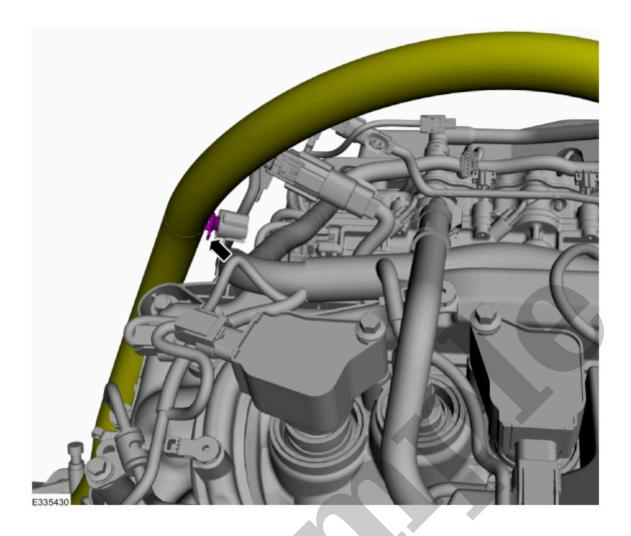
21. Install the ground strap and the nut to the RH (right-hand) valve cover stud bolt.
