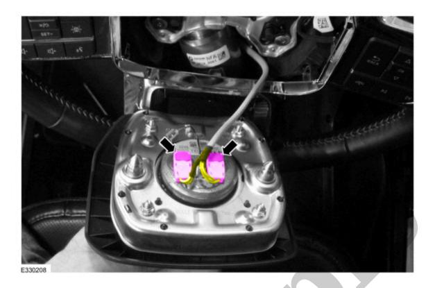
2. Align the driver airbag to the steering wheel and push in, engaging the driver airbag retainers to the spring clips.
