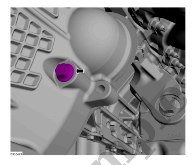
30. Remove the LH (left-hand) bellhousing bolt.
