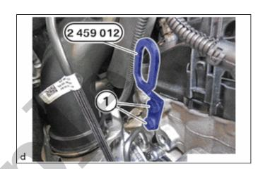
(b) Tighten the bolts (1) of special tool 2 459 012.
