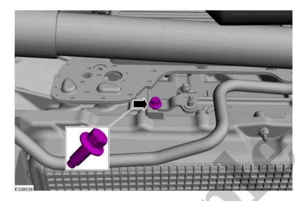
29. Remove the body-to-frame ground strap bolt RH (right-hand) frame bracket and position aside.
