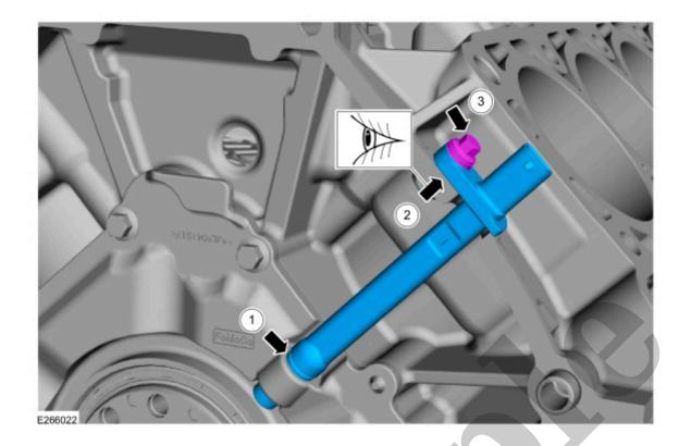
35. Install the crankshaft sprocket.
