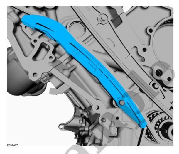
Install the RH (right-hand) timing chain tensioner arm.
