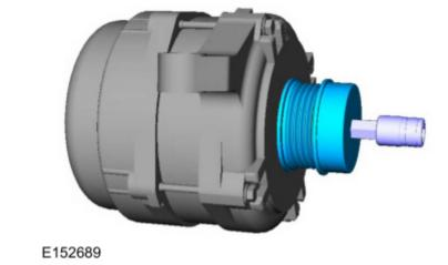
• While holding the clutch pulley firmly by hand, turn the clutch shaft clockwise. The clutch shaft should rotate smoothly and freely.
