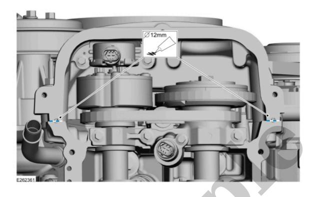
101. Install the valve cover and tighten the bolts.
