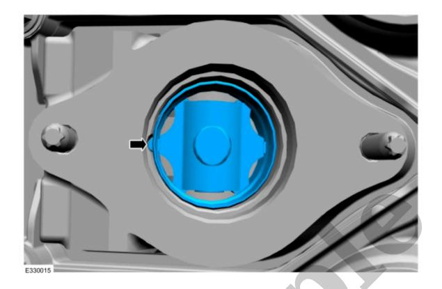
115. Install a new high-pressure fuel pump O-ring seal. Lubricate with clean engine oil.
