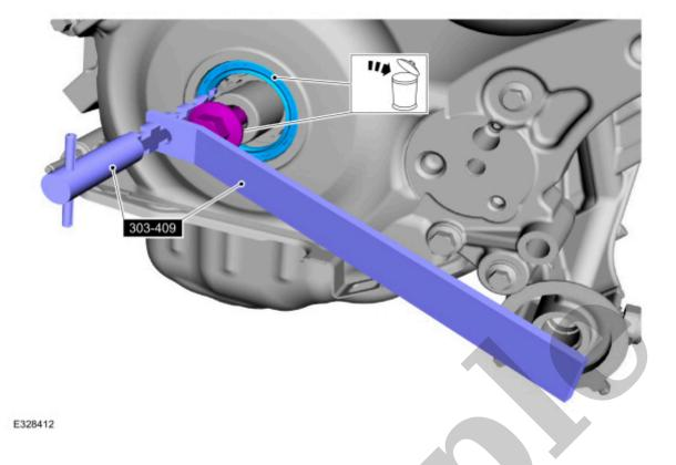
44. Remove the bolts and the coolant pump.
