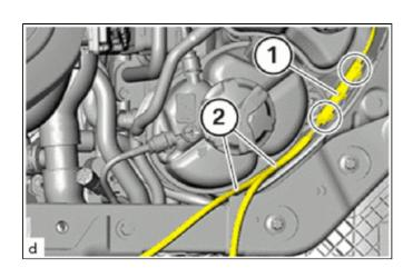
(d) Detach the Bowden cables (2) at the separation point in the housing (1) where required.
