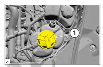
(b) Check the coolant level in the radiator reserve tank assembly for the high-temperature coolant circuit and top up the coolant where required.
