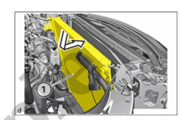
(b) Make sure the radiator assembly (1) is positioned correctly in the brackets in the marked areas.
