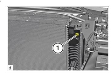
(f) Slightly pivot the radiator assembly (1) in direction of arrow and thread out and remove to the top.
