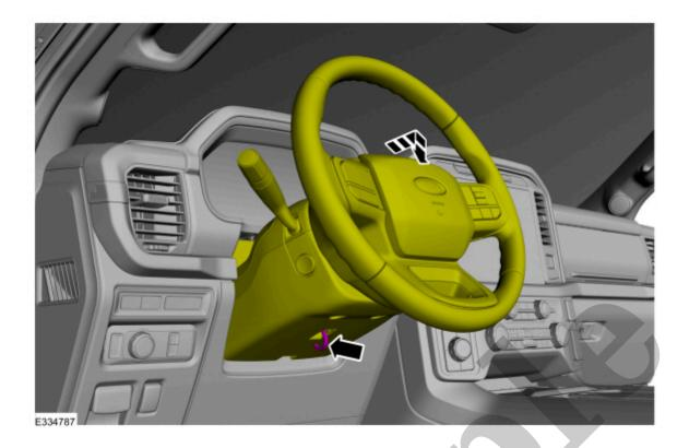
7. Release the tabs and disconnect the gap hider from the upper steering column shroud.
