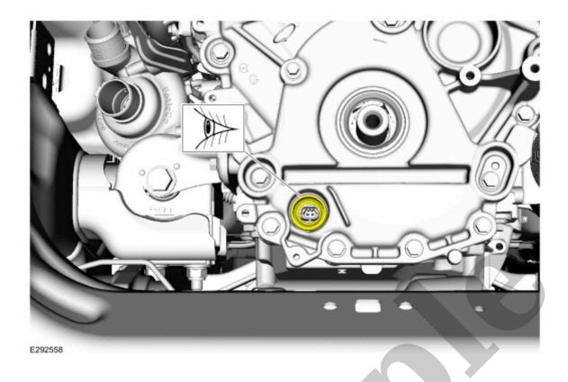
12. Install the transmission cooler bracket stud.
