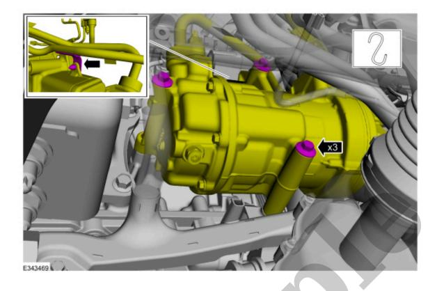
15. Remove the bolt and position the wire harness bracket.
