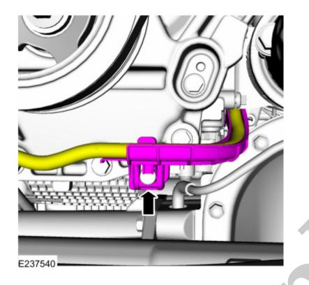
35. Detach the generator wiring harness retainer from the engine block.
