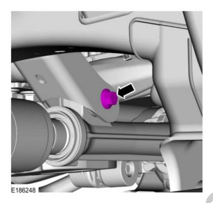
18. Tighten the upper front axle carrier mounting bushing bolt.
