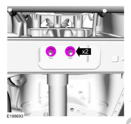
33. Position the exhaust Y-pipe dual catalytic converter-to-exhaust intermediate pipe and install the bolts.
