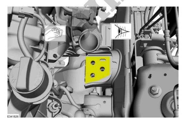
10. Hand start the new engine mount-to-frame bolts. Do not torque at this time.
