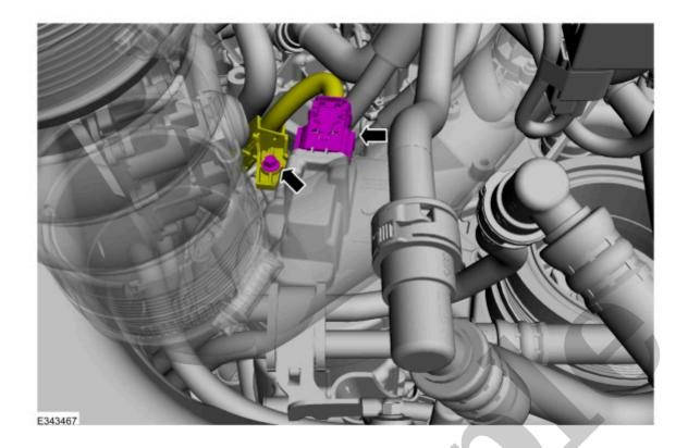
13. Disconnect the A/C (air conditioning) compressor electrical connector.
