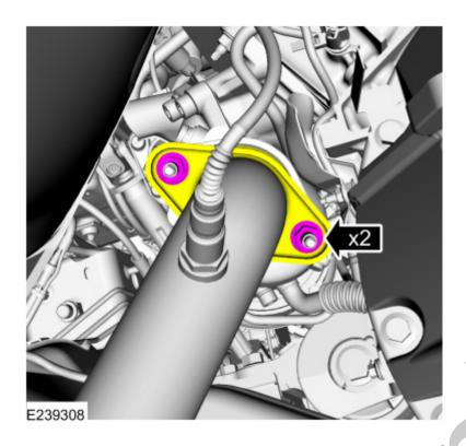
36. If equipped, install the front driveshaft.
