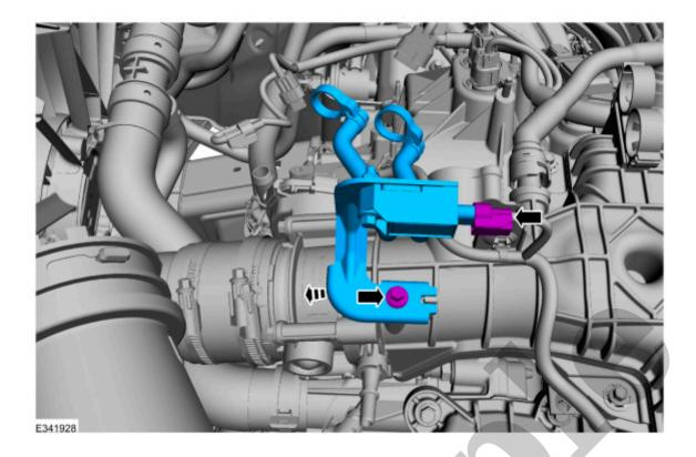
6. Disconnect the throttle body electrical connector and wiring harness retainers.
