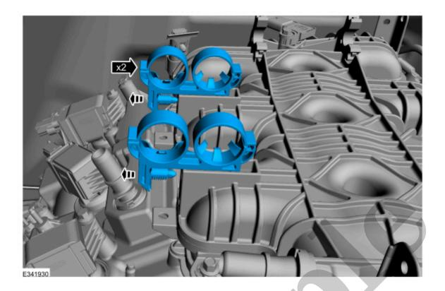
13. Remove the bolts and the intake manifold.
