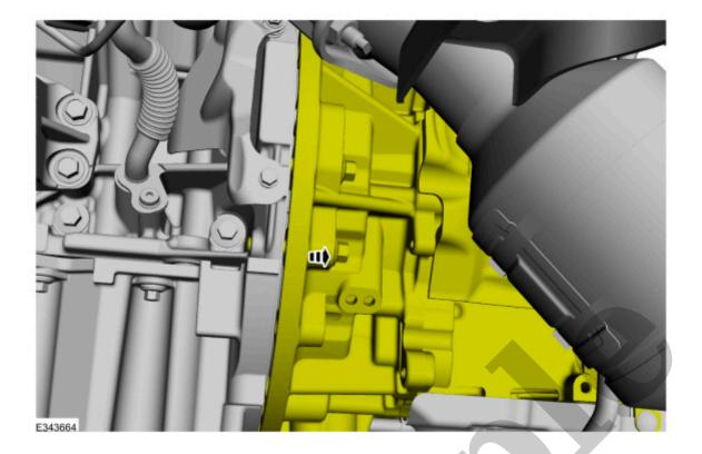
34. Remove the engine front cover bolts.
