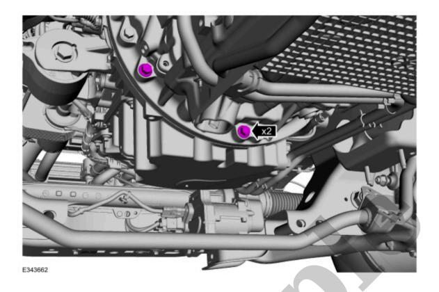
31. Loosen the bellhousing bolts 5 mm (0.19 in).
