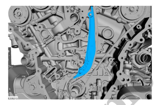
16. Remove the LH (left-hand) timing chain.
