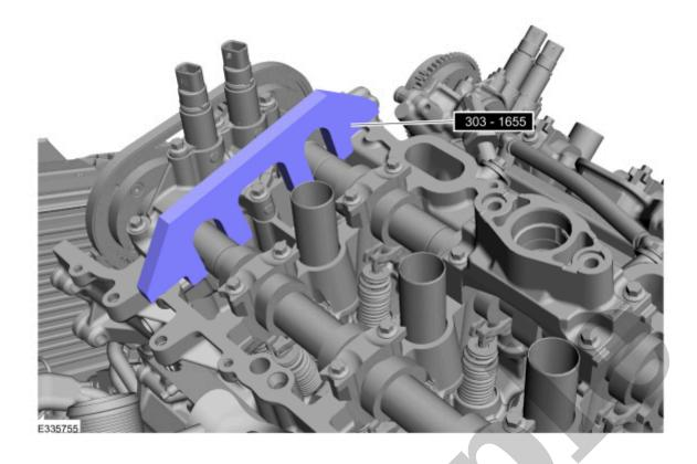
11. *Install Special Service Tool* : 303-1655 Tool, Camshaft Holding
