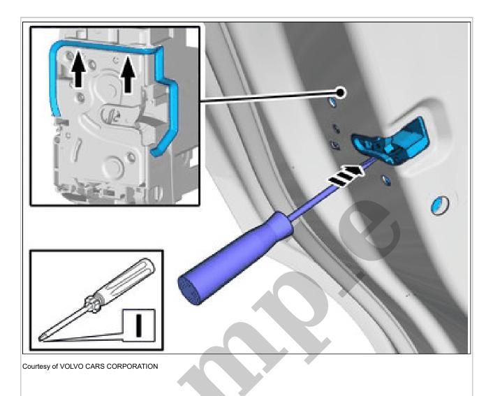
**CAUTION:** Lightly press the door latch so that the sealing is in the correct position.
