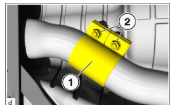
(j) Center the tail No. 1 exhaust pipe clamp (1) and tighten the nuts (2).
