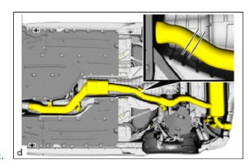
(b) Detach the exhaust pipe with the special tool 0 496 469 (00 2 220) at the separation point.
