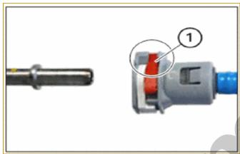
• Push fuel line (2) and fuel line (1) together in direction of arrow until both locks are heard to lock.
