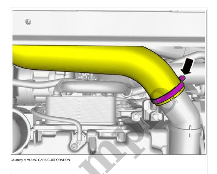
Loosen the hose clamp. Loosen the component indicated. Do not remove it.
