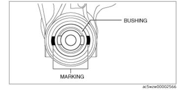
2. Press the rear hub support bushing (rear) out using the SSTs.
