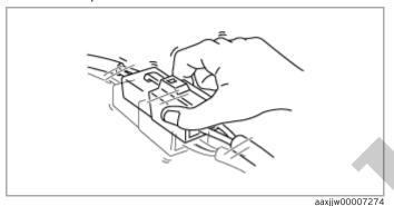
— Inspect the female terminals on the connector of the electric component which is suspected to be the cause of the malfunction for poor connection. (See **ELECTRICAL SYSTEM**.)
