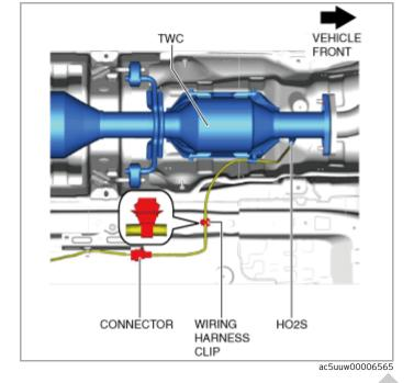
(2)Remove the TWC. (See EXHAUST SYSTEM REMOVAL/INSTALLATION [SKYACTIV-G 2.5 (WITHOUT CYLINDER DEACTIVATION)].) (See EXHAUST SYSTEM REMOVAL/INSTALLATION [SKYACTIV-G 2.5T].)
