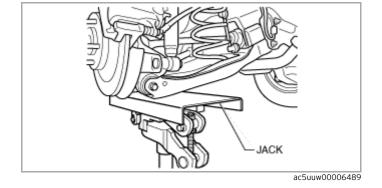
5.Install the rear lower arm outer bolt.
