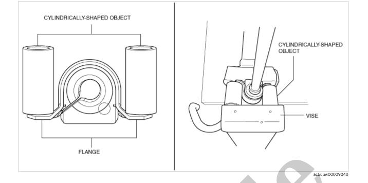
4.During rear stabilizer bracket installation, keep the deviation in the positions of the rear stabilizer bracket and the rear stabilizer bushing within the range shown in the figure.
