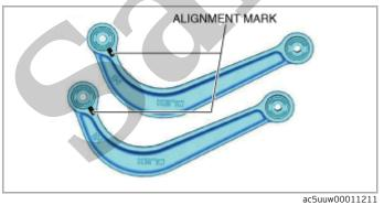
1. Align the alignment marks and tighten the rear upper arm inner bolt to the specified torque.
