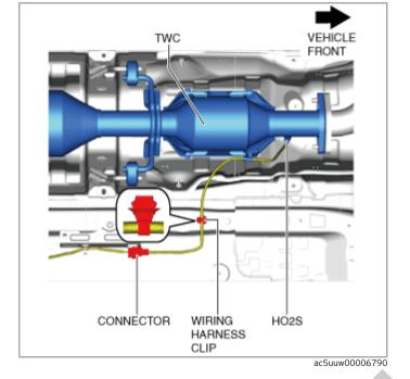
(4)Remove the TWC. (See EXHAUST SYSTEM REMOVAL/INSTALLATION [SKYACTIV-G 2.5 (WITH CYLINDER DEACTIVATION)].)
