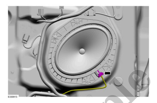
3. Remove the screws and the front door speaker.
