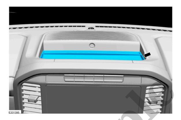
2. Release the clips and remove the center instrument panel speaker grille.
