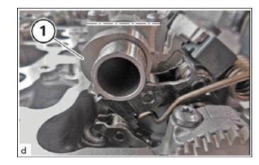
(e) Ensure that the flattened areas (1) on the intake camshaft subassembly and the exhaust camshaft sub-assembly point upwards.
