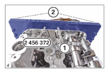
(f) Position the basic carrier (1) from the set of special tools 2 456 372 on the cylinder head sub-assembly.
