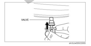
4.Install the valve removal tool to the air pressure sensor valve.
