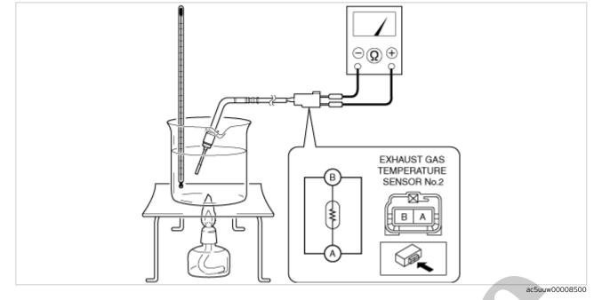
• If not as specified, replace the exhaust gas temperature sensor No.2. (See EXHAUST GAS TEMPERATURE SENSOR REMOVAL/INSTALLATION [SKYACTIV-D 2.2].)
