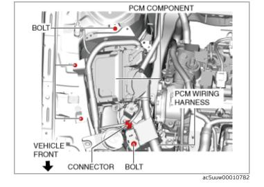
(3)Move the PCM component in the direction of the arrow shown in the figure and set it aside with the PCM connectors connected.
