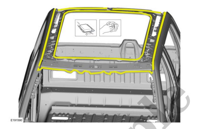
3. Sand to remove any remaining adhesive in the rear flange and clean.
