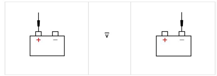
Is the recorded battery voltage within ±0.5 volt of the PID (parameter identification)?
