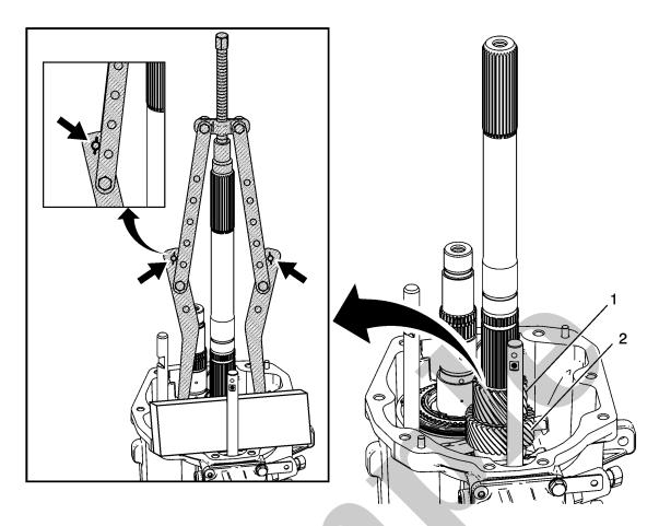
7th Driven Gear and 5th Driven Gear Removal-Stage 1
