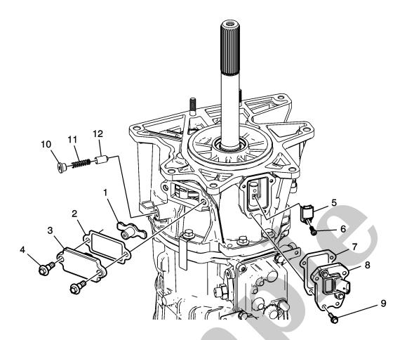
7th/Reverse Inverter Link Cover and Gear Position Sensor Installation
