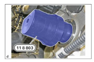
(i) Screw on the special tool (nut) 0 496 131 (11 8804) until the special tool (sleeve) 0 496 130 (11 8803) lies flush on the cylinder block sub-assembly.
