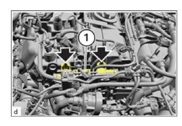
(r) Connect and lock all connectors (1) in the direction of the arrow.
