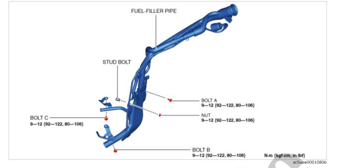
2.Temporarily tighten bolt A.
