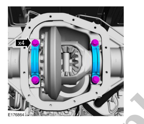
7. Remove the differential carrier, differential carrier bearing cups and the differential shims.
